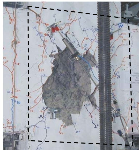
Figure 14: Laboratory testing of OMF sub-assembly (see Figure 1). Here, concrete has spalled in the beam-column joint region (outlined by dashed line) exposing column longitudinal reinforcing steel (Lehman et al. 2002).
