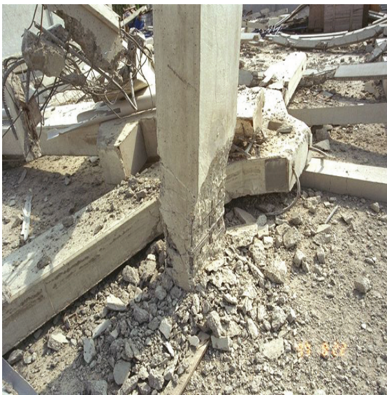
Figure 13: Severe spalling of column cover concrete exposing longitudinal steel. Damage resulted from Izmit earthquake. Image by H. Sezen (1999), courtesy of National Information Service for Earthquake Engineering, EERC, UC Berkeley.
